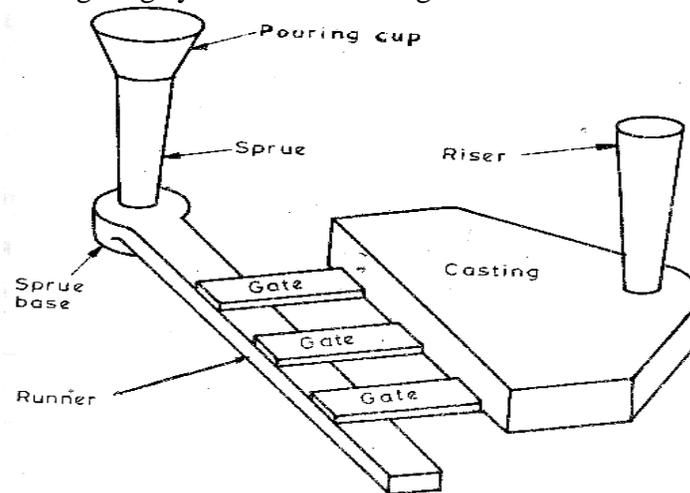
Since the way which liquid metal enters the mold has a decided influence upon the quality and soundness of a casting, the different passages for the molten metal are carefully designed and produced. A gating system should avoid sudden or right angle changes in direction. Sudden change in direction causes mold erosion, turbulence and gas pick up. If possible the gating system should form a part of the pattern. It
