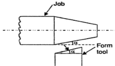
Fig. Taper turning by a form tool.
