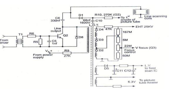
Anode potential (G2) is obtained for screen grid separately at collector of Q2
